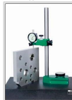
rigid construction, designed to make comparison height measurement (set zero with gage block then measure height of workpiece) with dial indicators or electronic indicators (variation of measuring force is high)
