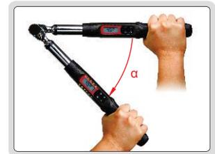
Set the desired torque first. After reaching the desired torque, set the angle and turn the wrench at this angle to apply extra torque
