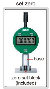
measure peak-to-valley height of blast cleaned surfaces
